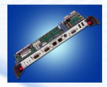
This single-slot, 6U board provides rear panel access to the I/O functions of an IPnexus™ single board computer (SBC) with RPIO-pin compatibility, such as the IPnexus ZT 5504e System Master Processor Board. It is also designed to function with other third-party PICMG® 2.16-compliant SBCs. The IPnexus ZT 4807e easily snaps into the rear panel slot of a 6U PICMG 2.16-compliant CompactPCI® system such as the IPnexus ZT 5091e 4U Packet-Switched Platform.
