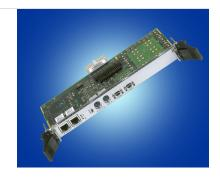
This 6U, single-slot rear panel transition board provides rear panel access to the I/O functions of a number of Performance Technologies' single board computers (SBC) - specifically the ZT 5503. The ZT 4806 is designed to function in the rear panel slot of a CompactPCI® system that accepts 6U boards, such as the ZT 5087e 4U General Purpose Platform.
