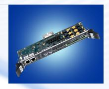
This 6U, single-slot, rear panel transition board with alarm outputs provides rear panel access to the I/O functions of a number of Performance Technologies single board computers (SBC), specifically the ZT 5503 and ZT 5551. It is designed to function in the rear panel slot of several Performance Technologies 6U CompactPCI® systems and enclosures, providing interfaces for two user inputs and six alarm relay outputs.
