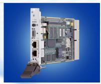
Shelf management ensures maximum service availability in a computing platform by monitoring sensors and predicting failures. The CPC7301 Intelligent Shelf Manager offers a comprehensive management architecture that delivers high availability protection with reliable, redundant and IPMI (Intelligent Platform Management Interface) standards-based management to all the major components in the shelf, including the entire IPnexus<sup>™</sup> product family.
