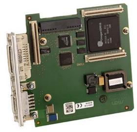
The P17 is based on the PC-MIP ANSI mezzanine standard. It can be used as an I/O extension in any type of bus system, i.e. CPCI, PXI, VME or on any type of stand-alone SBC. Appropriate PC-MIP carrier cards in 3U, 6U and other formats are available from MEN or other manufacturers. Comparable with the larger foot print PMC mezzanine cards, PC-MIP boards also support PCI bus.
