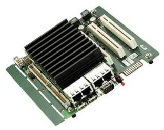
Embedded System Modules are complete computers on a module. A final application consists either of a standalone ESM, an ESM with an application-specific carrier card and/or an ESM with additionally plugged PCI-104 modules.
