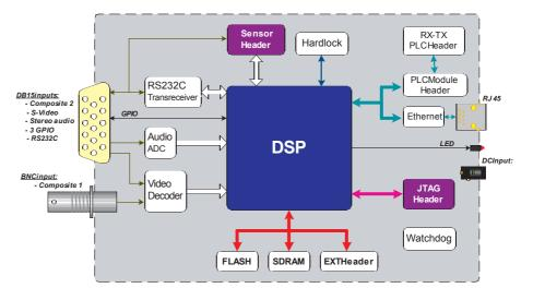
The DSP has a 32 MB SDRAM running at 100 MHz and 64 bits, which provides a throughput of 800 MB/s.
