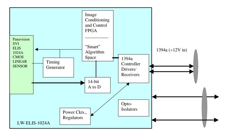
Optional External Sync Programmable I/O (with +5V, +12V out)
